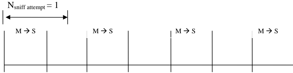
Figure 7: Anchor point with no communication from master
