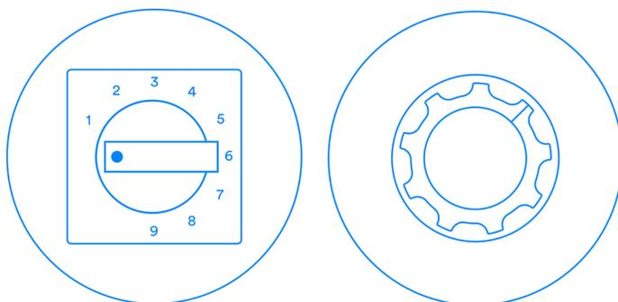
Figure 4a (left) - A 9 x Position Rotary Switch
