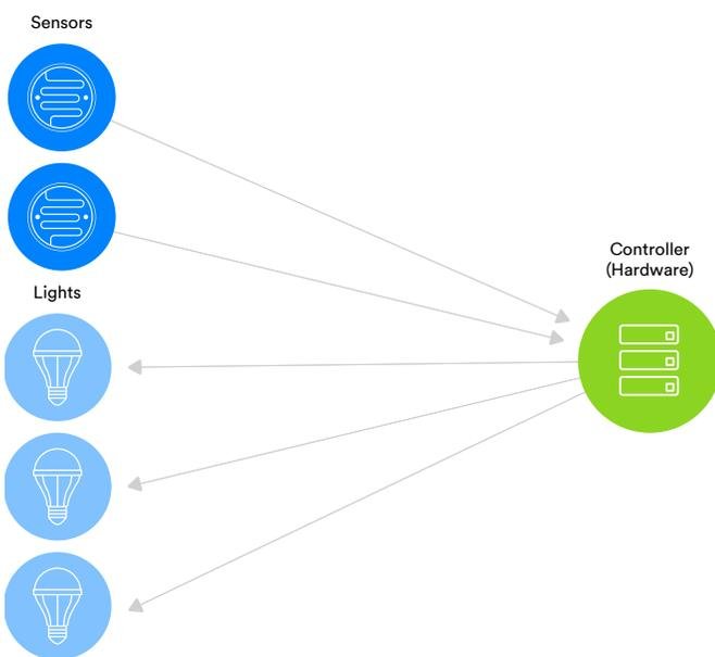
Figure 13 -The Lighting Models Legacy, Centralized Lighting Control
