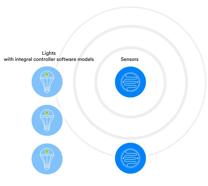
Figure 14 -The Bluetooth Mesh Decentralized Controller Architecture
